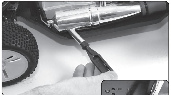
4. Stopping the engine. To stop the engine either use a stop tool to cover the exhaust outlet or use a flywheel stop tool.
